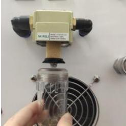
c. After the operation, discharge the gas until the water in the center is back to position 0 automatically in the cup. Remove it if necessary Clean, rotate to the left, and pay attention to the black sealing ring of the filter cup when installing.
