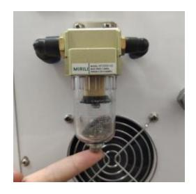
b. Turn to the left and unscrew the filter cup, pour out the water inside and rinse and dry it with clean water.
