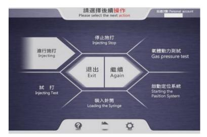
Enter the syringe inter face, take out the syringe and extract the liquid again. Follow the previous steps to turn off the gas main switch and pull he handle trigger to release the gas in the table and in the trachea Come out, and finally turn off the power switch and rotate to release the pressure adjustment button.
