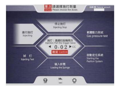
2) Continuous mode: select the dose according to the demand, and click the confirmation button, you can continuously pull the trigger for operation.
