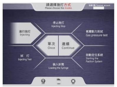
1) Single mode: select the dose according to the requirements, click the confirmation button to start the operation, and pull the trigger twice each time Re-click the confirmation button.
